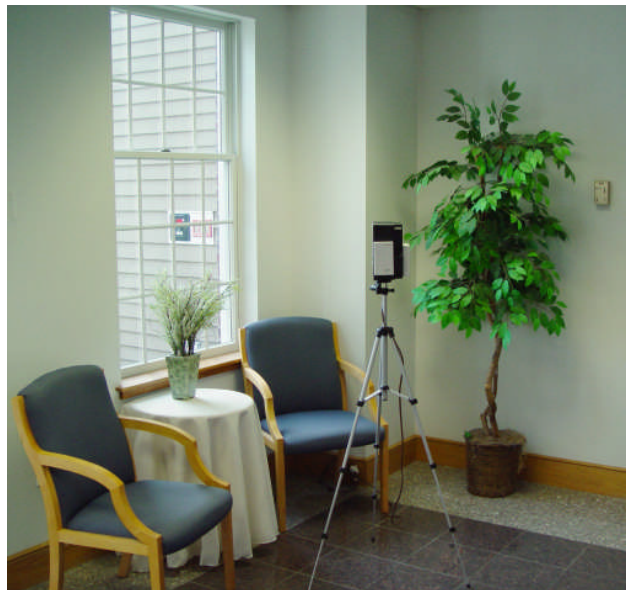
Spinwave's wireless indoor monitor can be placed anywhere in a building to monitor temperature, relative humidity, and CO 2 levels.
